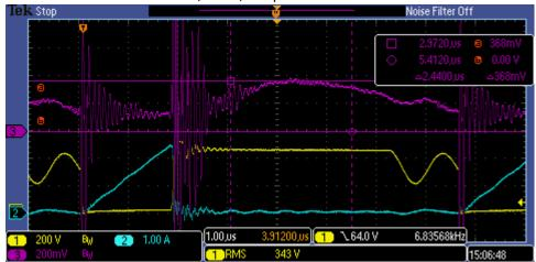
"Bad" TOPSWITCH: 3A load, 240V, the peak feedback current comes to ~8.2mA.
