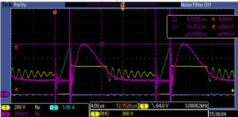
CH1: drain voltage, CH2 drain current, CH3 feedback current ( $100\Omega$  emitter of OP1)
