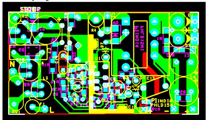
Note: All three input drum inductors need to be modified to 10x12 size from the present 8x10
