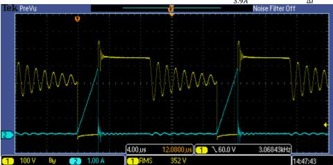
The default current limit for the TOP270 is 5.17A. The current limit is set to  $^{\sim}4.76A$  which is 92% of the default limit by using R6 = 8k2. The current limit from which the PSU enter the variable frequency area is the limit kPS(upper) = 55% of the current limit set.  $2.62A = 55\% \times 92\% \times 5.17A$
