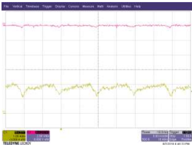
Figure 27 – Main Output Voltage and Current Ripple in CC Mode, 180 VAC, Chroma CV Load, 30 V Setting. Upper: Main V_{OUT(RIPPLE)} , 2 V / div. Lower: I_{OUT(RIPPLE)} , 1 A, 5 ms /div.
