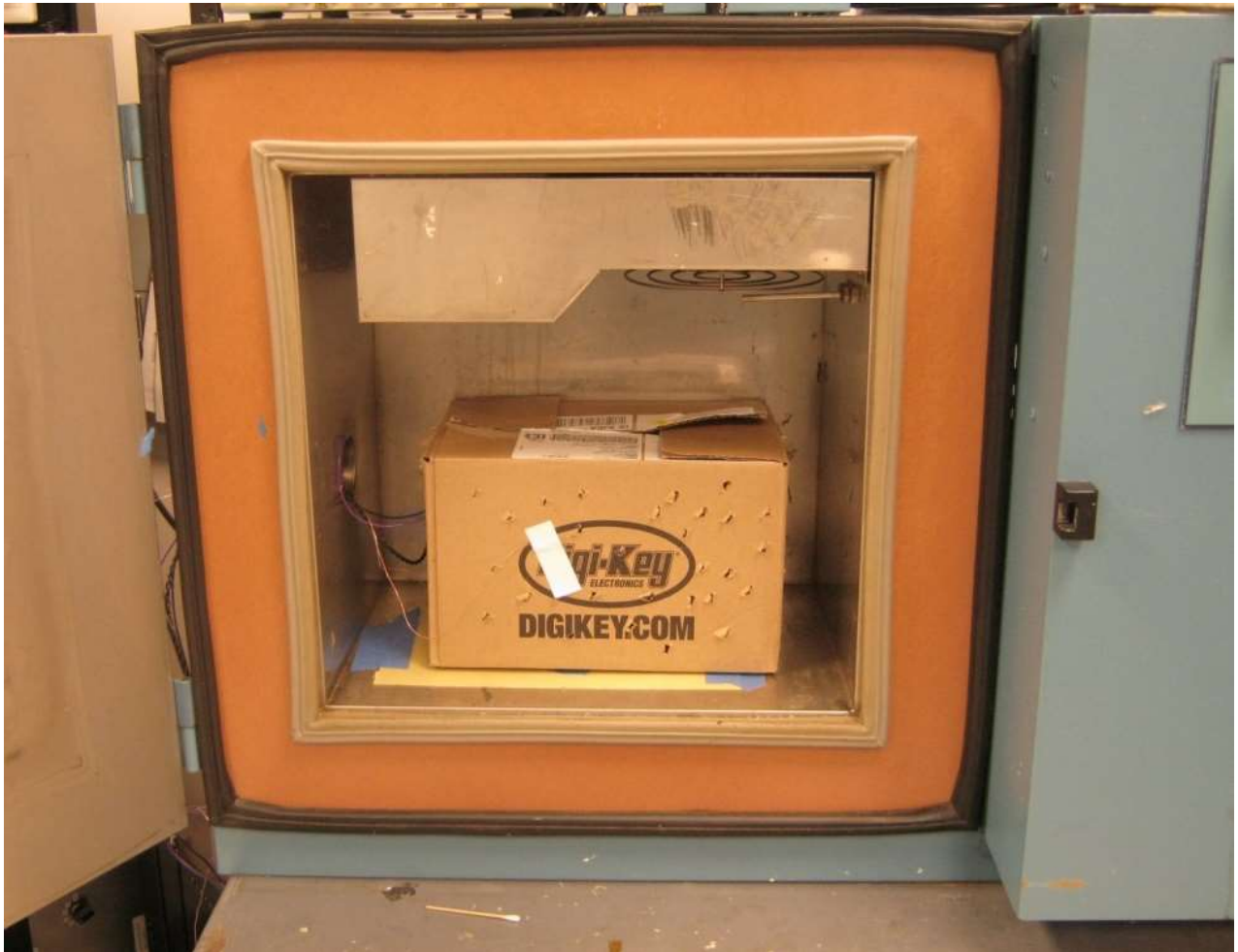
Figure 33 – Isolation Box in Thermal Chamber.
