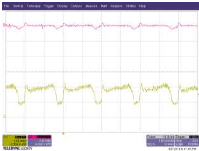
Figure 25 – Main Output Voltage and Current Ripple in CC Mode, 180 VAC, Chroma CV Load, 57 V Setting. Upper: Main V_{OUT(RIPPLE)} , 2 V / div. Lower: I_{OUT(RIPPLE)} , 1 A, 5 ms /div.
