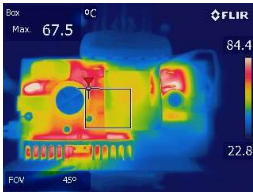
Figure 34 – Top View Thermal Picture, 165 VAC.
