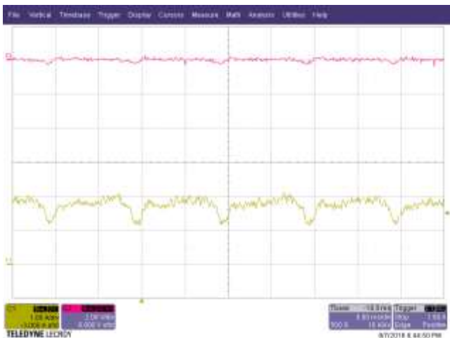
Figure 28 – Main Output Voltage and Current Ripple in CC Mode, 230 VAC, Chroma CV Load, 30 V Setting. Upper: Main V_{OUT(RIPPLE)} , 2 V / div. Lower: I_{OUT(RIPPLE)} , 1 A, 5 ms /div.
