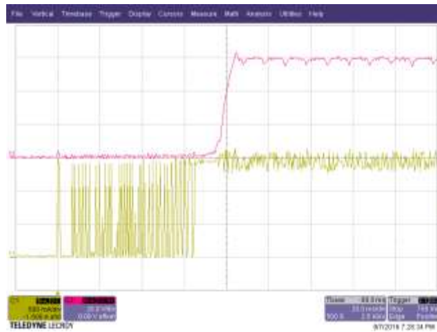
Figure 17 – Output Start-up, CV Mode, 230 VAC, Chroma CC Load, 1.5 A Setting. Upper: V_{OUT} , 20 V / div. Lower: I_{OUT} , 0.5 A, 20 ms / div.
