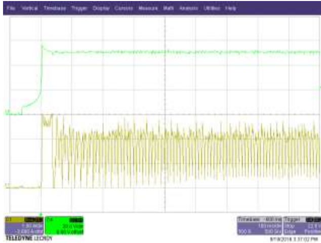
Figure 18 – Output Start-up, CC Mode, 230 VAC, Chroma CV Load, 50 V Setting. Upper: Main V_{OUT} , 20 V / div. Lower: Main I_{OUT} , 1 A, 100 ms / div.
