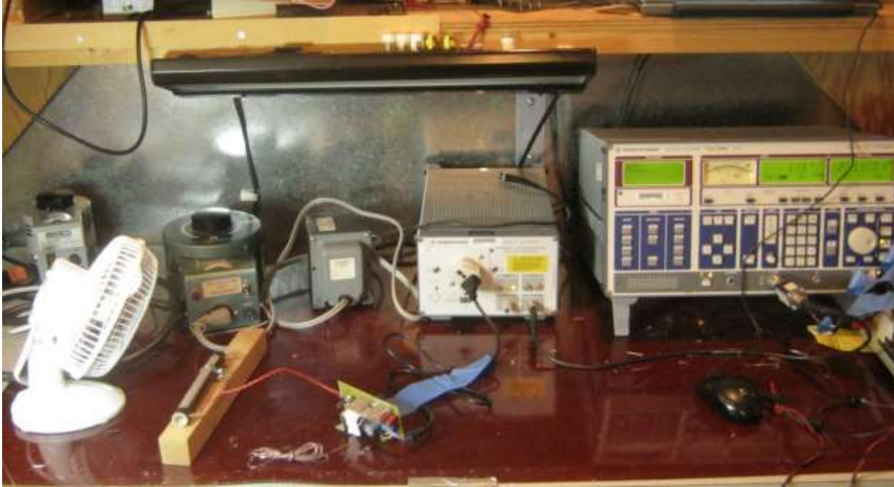
Figure 38 – EMI Set-up with Floating Resistive Load.
