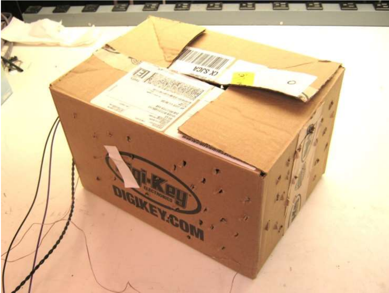
Figure 32 – Isolation Box with Equilibration Holes for Thermal Chamber Testing.
