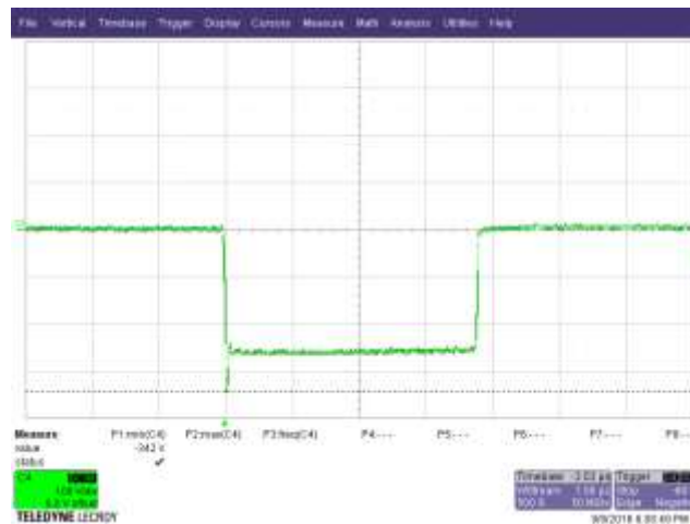
Figure 16 – Output Rectifier (D3) Reverse Voltage, 230 VAC Input, 100% Load. 100 V, 1 \mu s / div.
