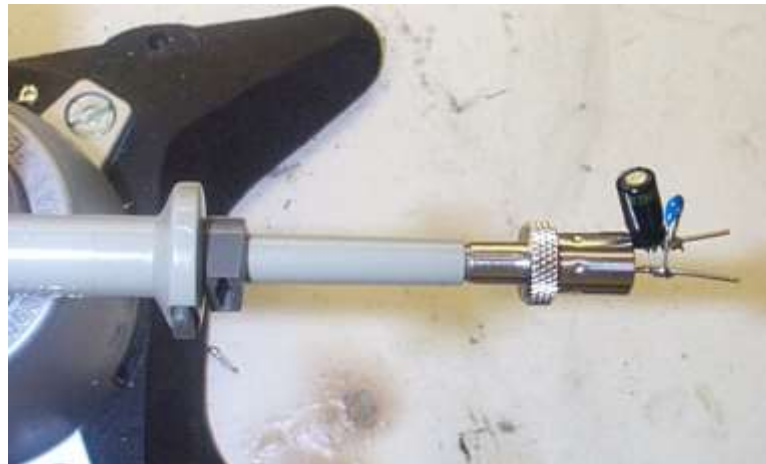
Figure 22 – Oscilloscope Probe with Probe Master 4987BA BNC Adapter (Modified with Wires for Probe Ground for Ripple measurement and Two Parallel Decoupling Capacitors Added).
