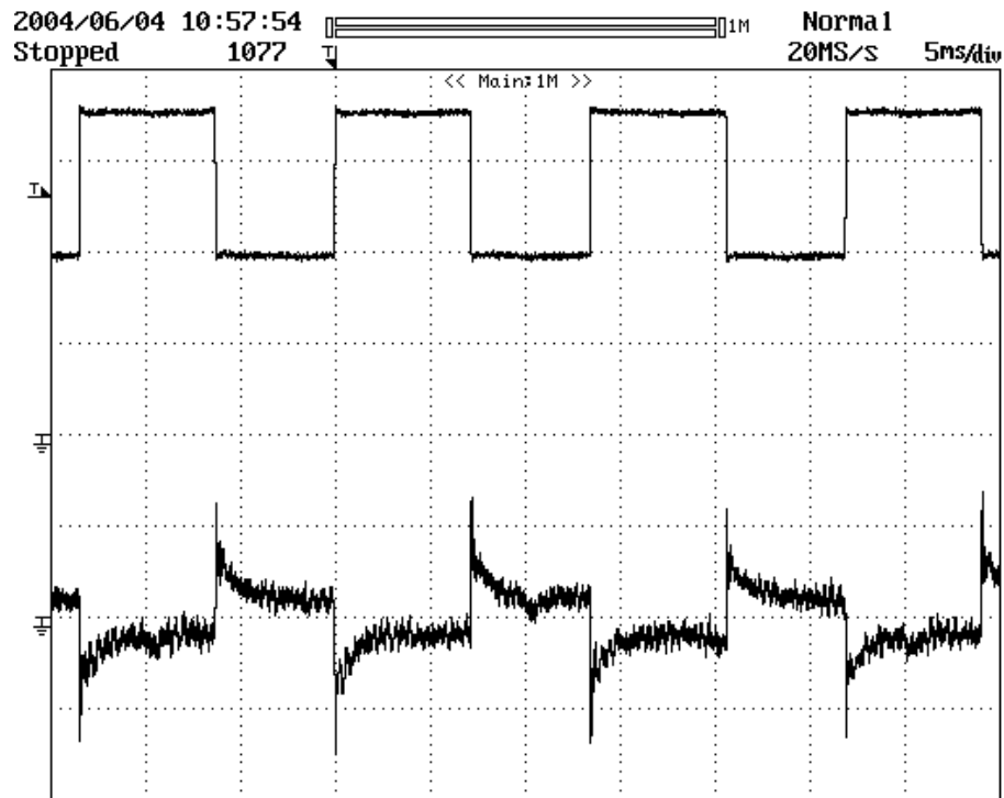
Figure 17 – Transient Response, 230 VAC, 0.4A to 0.75A Current Change on 3V3 output. Top: 3V3 Rail Current, 0.2 A/div. Bottom: AC Coupled 3V3 Rail Output Voltage 50 mV, 5 ms / div.
