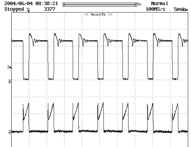
Figure 10 - 265 VAC, Full Load Lower: I_{DRAIN} , 0.2 A / div Upper: V_{DRAIN} , 200 V / div
