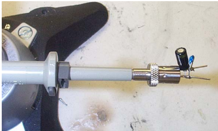
Figure 10 – Oscilloscope Probe with Probe Master 5125BA BNC Adapter. (Probe modified with wires for probe ground, and two parallel decoupling capacitors added).
