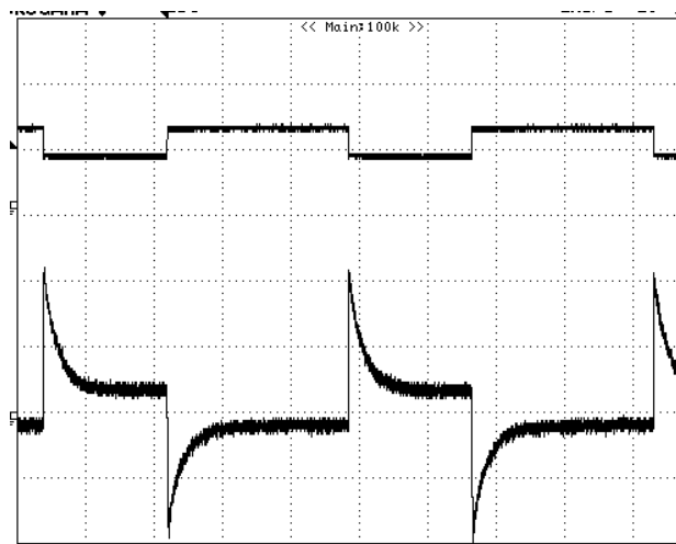
Figure 20 – Transient Response, 230 VAC, 100-50% Load Step. Upper: Load Current, 0.5 A / div. Bottom: Output Voltage 200 mV, 10 ms / div.
