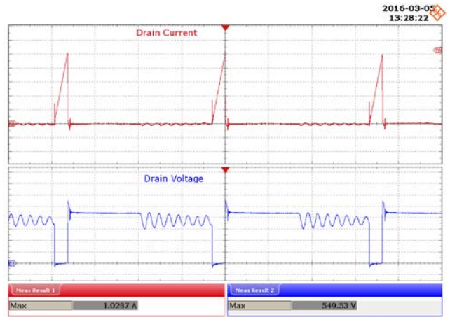
Figure 87 – 265 VAC, 20 V LED Load. Upper: I_{DRAIN} , 200 mA / div. Lower: V_{DRAIN} , 100 V / div., 4 μs / div.
