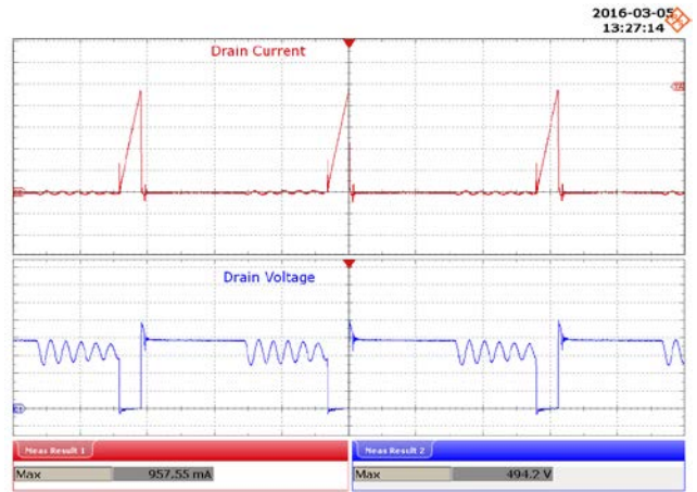
Figure 85 – 230 VAC, 20 V LED Load. Upper: I_{DRAIN} , 200 mA / div. Lower: V_{DRAIN} , 100 V / div., 4 μs / div.
