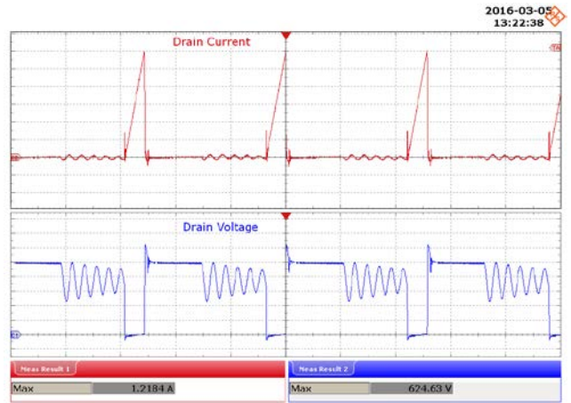
Figure 79 – 265 VAC, 40 V LED Load. Upper: I_{DRAIN} , 200 mA / div. Lower: V_{DRAIN} , 100 V / div., 4 \mu s / div.
