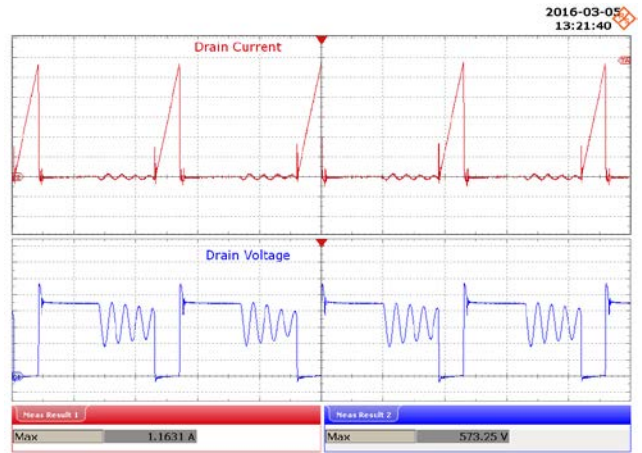
Figure 77 – 230 VAC, 40 V LED Load. Upper: I_{DRAIN} , 200 mA / div. Lower: V_{DRAIN} , 100 V / div., 4 \mu s / div.
