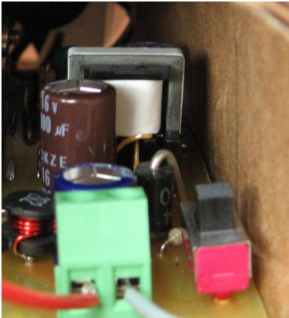
Figure 54 – Standby Transformer T2, Visible Light View.
