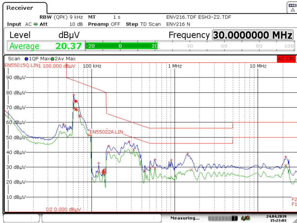
Figure 84 – Conducted EMI QP Scan at 42 V LED Load, 230 VAC, 60 Hz, and EN55015 B Limits.
