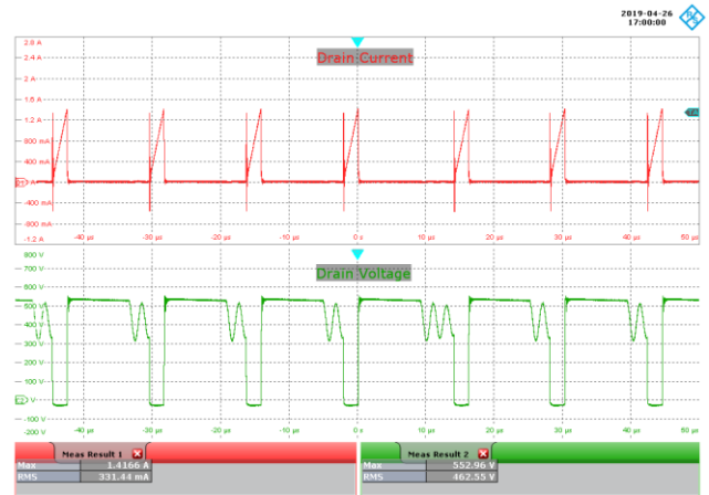
Figure 70 – 265 VAC, 42 V LED Load. Upper: I_{DRAIN} , 400 mA / div. Lower: V_{DRAIN} , 100 V / div., 10 \mu s / div.
