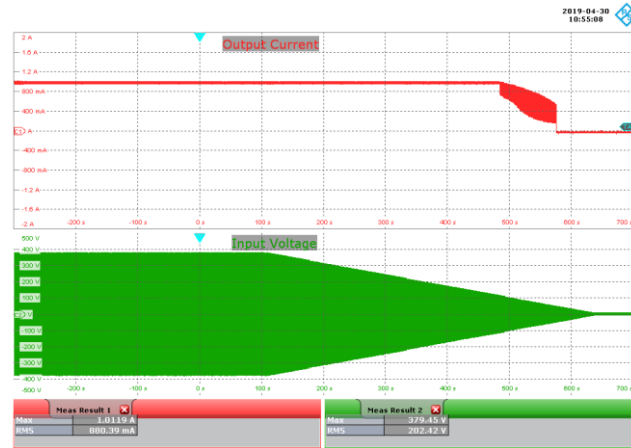
Figure 87 – Brown-out Test at 0.5 V / s Ch1: I_{OUT} , 400 mA / div. Ch2: V_{IN} , 100 V / div. Time Scale: 100 s / div.
