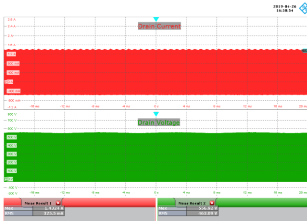
Figure 67 – 230 VAC, 42 V LED Load. Upper: I_{DRAIN} , 400 mA / div. Lower: V_{DRAIN} , 100 V / div., 4 ms / div.
