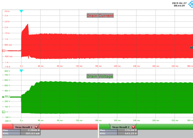
Figure 71 – 198 VAC, 42 V LED Load. Upper: I_{DRAIN} , 400 mA / div. Lower: V_{DRAIN} , 100 V / div., 40 ms / div.
