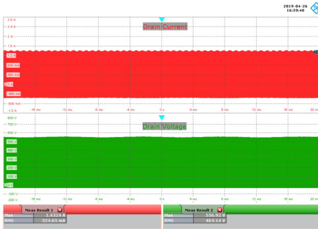
Figure 69 – 265 VAC, 42 V LED Load. Upper: I_{DRAIN} , 400 mA / div. Lower: V_{DRAIN} , 100 V / div., 4 ms / div.
