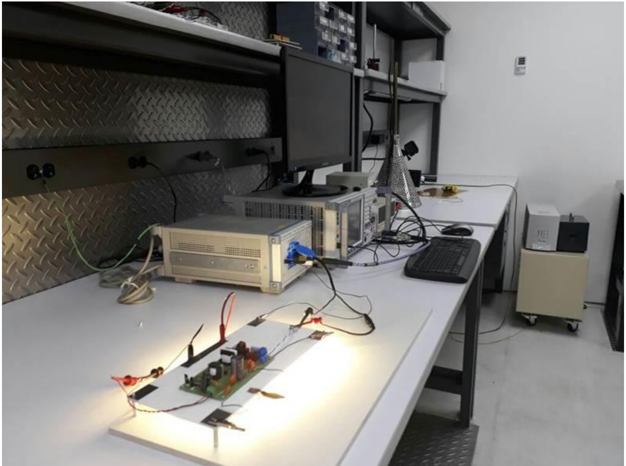
Figure 83 – Conducted EMI Test Set-up.
