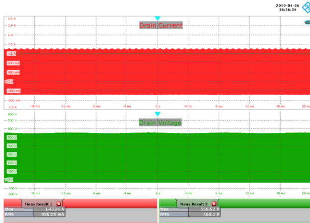
Figure 65 – 198 VAC, 42 V LED Load. Upper: I_{DRAIN} , 400 mA / div. Lower: V_{DRAIN} , 100 V / div., 4 ms / div.
