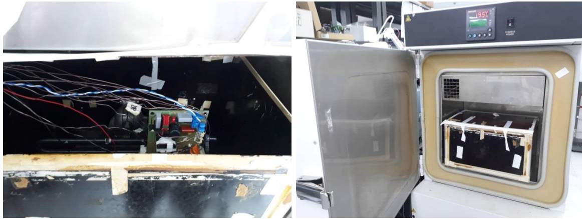
Figure 36 – Test Set-up Picture Thermal at 60 °C Ambient - Open Frame.
